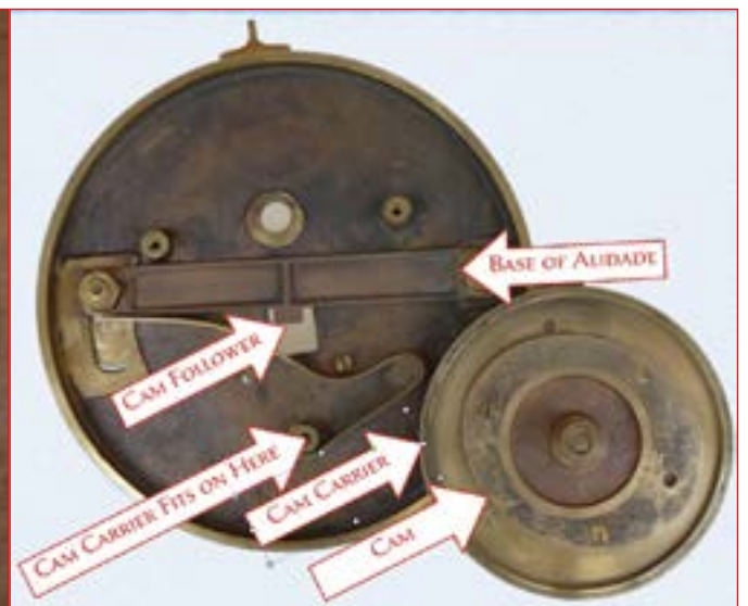
the mechanical working of a Pilkington Gibbs - showing the cam and its follower, which is attached to the alidade .
