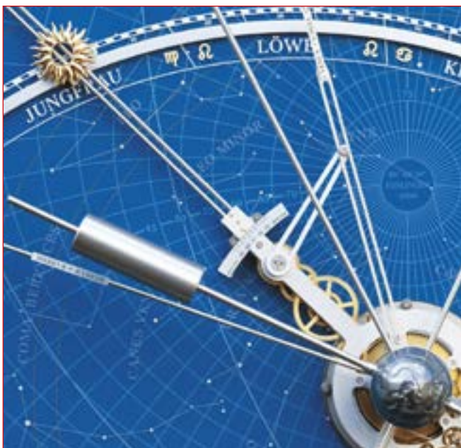
Face detail, showing Solar Hand and EoT Indicator
