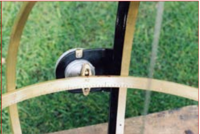
Inner cam carrying an eccentric pin driving the Hour ring.
