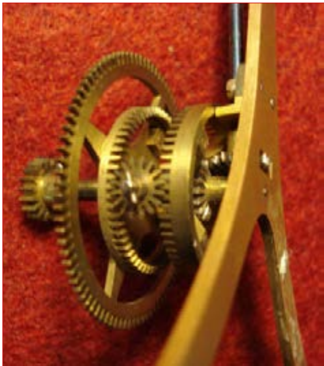
A differential adder from the 1930's Astronomical Clock by Paul Pouvillon
