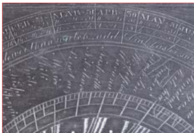
Fig. 13. Part of the EoT ring on a multiple-gnomon slate dial by Richard Melville. This Sussex dial, from relatively late in Melville's career, has the correct value of 4 mins for May 20. Photo: Harriet James
