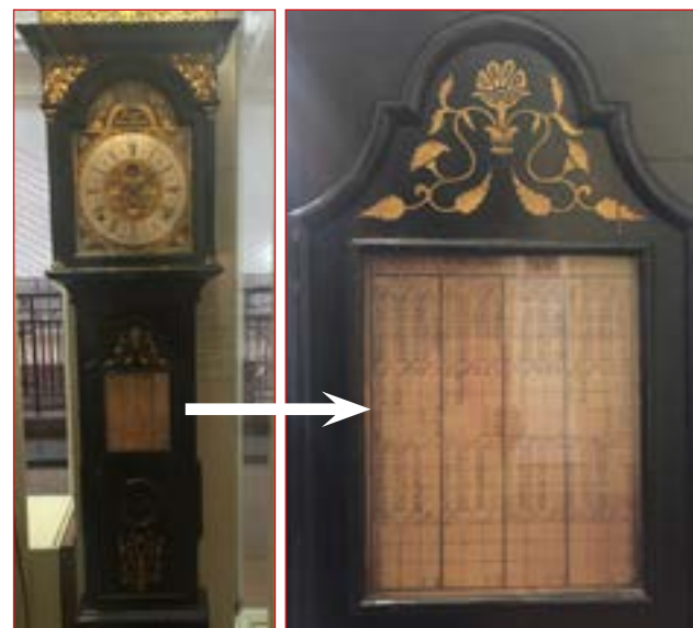
One of two of John Harrison's personal regulators, with Equation Table in his own hand, printed on pendulum door. This clock was set, not by the sun, but by the stars viewed between Harrison's door post and his neighbour's chimney.
