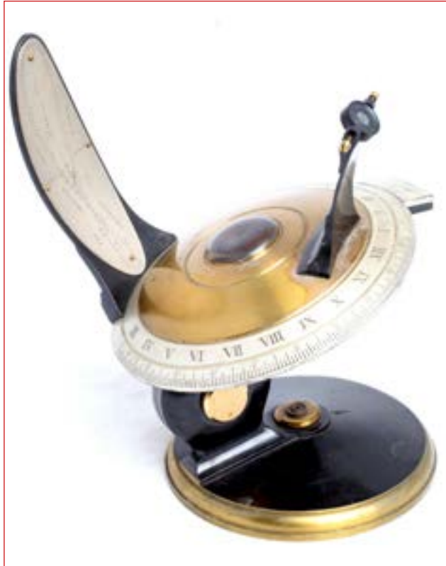
19th C, French Heliochronometer by Radiguet-Massiot, Paris - previously thought to have been used by the French Railways - but this is not the case..
