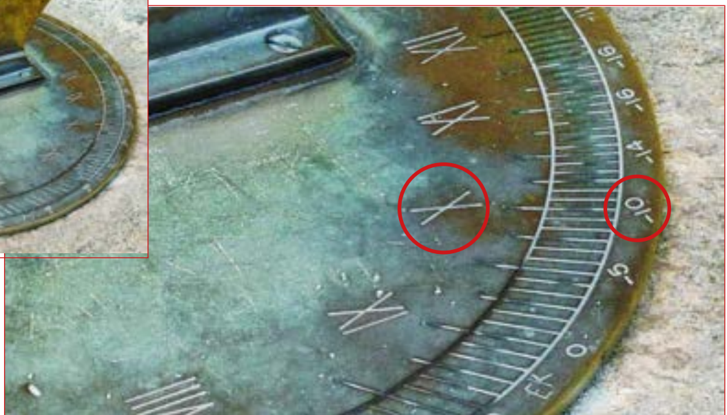
Kirstenbosch Botanical Gardens = 1920 - by J.R. Miller. EoT is marked around the rim of the dial in positions corresponding to the date in the month. Thus at the beginning of the 10th month (X) is -10 mins
