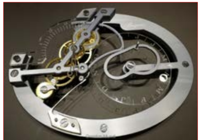
Breguet No. 160 "The Grand Complication," commonly known as the Marie-Antoinette. The cam is visible, but not the intermittent sampler.
