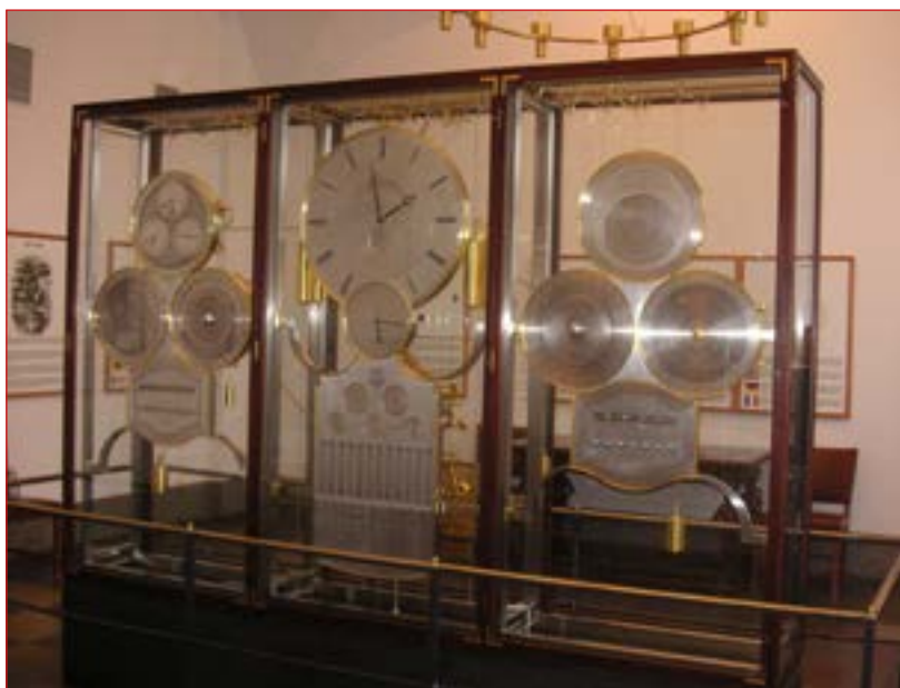
The Front of the Jens Olsen Clock. The top left face shows the Equation of Time, Local time and Solar Time.
