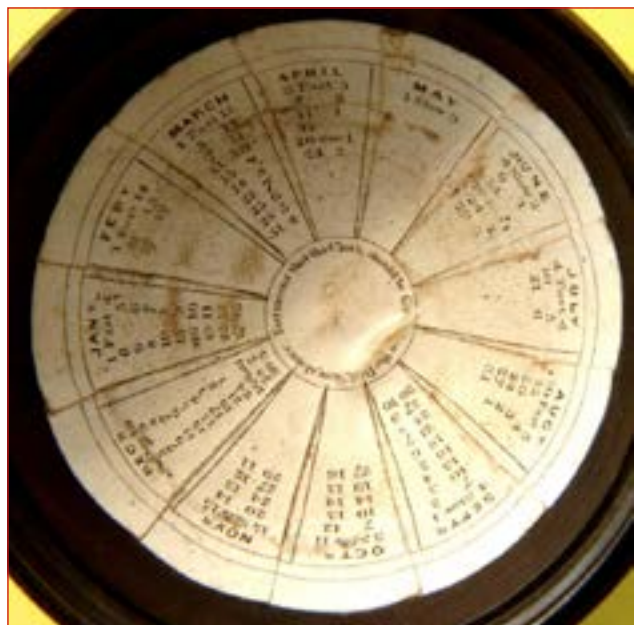
Fig. 7. An EoT table pasted into the lid of a magnetic compass dial. Photo: M. Cowham
