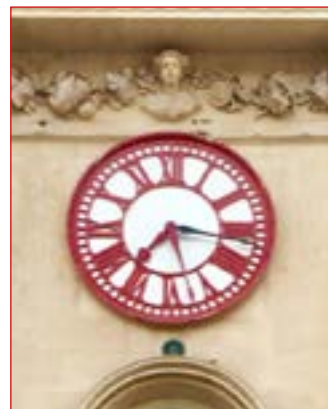
Bristol 1753 Corn Exchange Clock, showing Greenwich Mean Time and Bristol Mean Time (the black hand). Bristol local mean time at 2.5°W is 10 minutes behind Greenwich Mean Time
