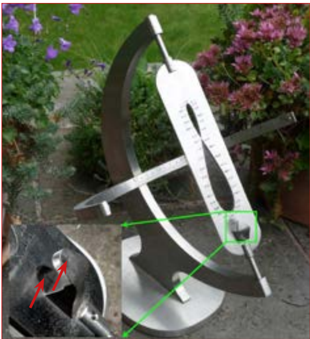
Tony Moss 'Henry Moore' dial - ca 2010 - note the clever arrangement to ensure that the plane of the analemma is perpendicular to the sun's rays
