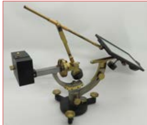
1862 - Heliostat, based on clockwork, built on a form devised by Leon Foucault. It required daily EoT correction.
