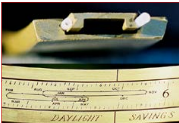
The sliding time strip in the helix of a Renaissance Dial, showing the EoT setting for either 29th September or 5th December (when they are the same)
