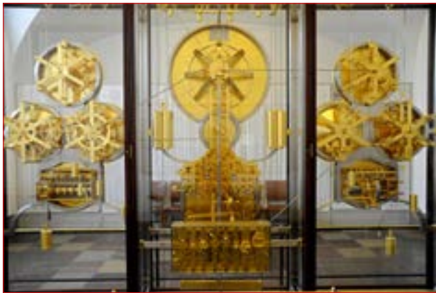
The Rear of the Jens Olsen Clock. The rectangular section (bottom centre) generated the 5 sine components of the lunar motion and, at the right, the 2 main & 1 small sine components of the Equation of Time. The connection between the signal generation and the Dial (now top right) is via a steel ribbon.
