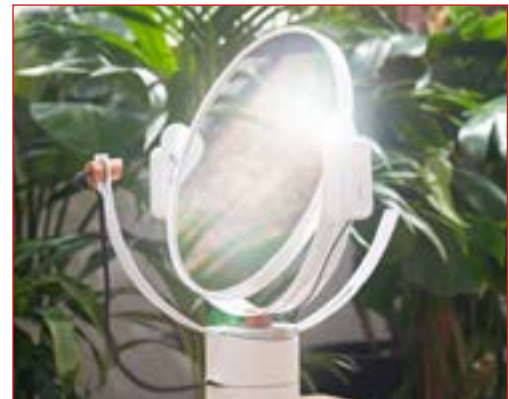
2023 - A beautiful Solenica heliostat by Diva Tommei - all driven by electronics, sensors & software. No need for the EoT!
