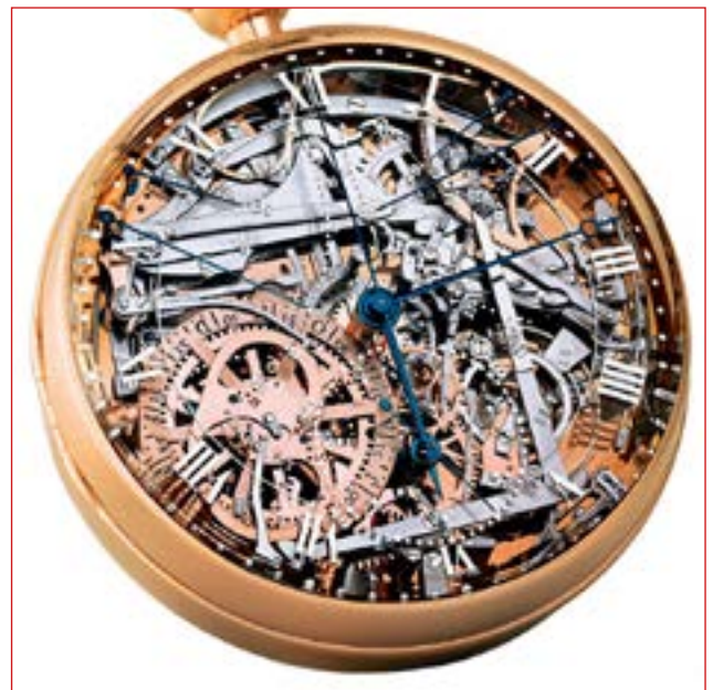
Breguet No. 160 "The Grand Complication," commonly known as the Marie-Antoinette. The cam is visible, but not the intermittent sampler.
