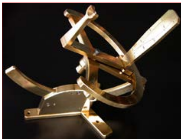
J.D Gard - Aten Heliochronometer - ca 2006 These dials used to be commercially available in bronze or aircraft-grade aluminium
