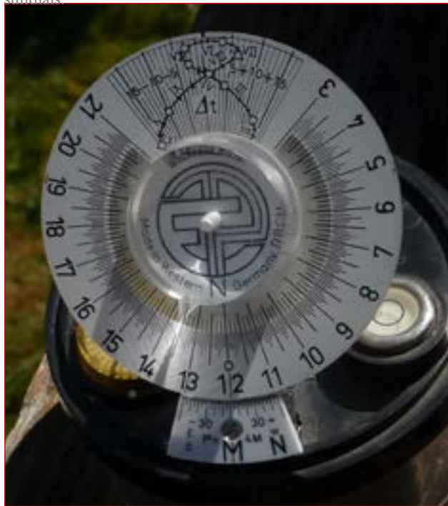
Fig 14 -Erich Pollähne's improved Benoy-Type sundial. Note how, instead of a shadow, the time is told by the cusp of light
