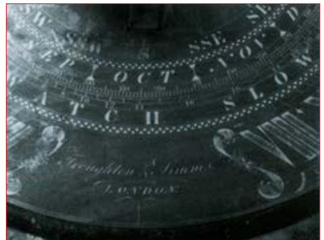
Figure 6: Part of the EoT ring on a late 19 th century dial by Troughton and Simms. The months are written anticlockwise so that the days increase left to right.
