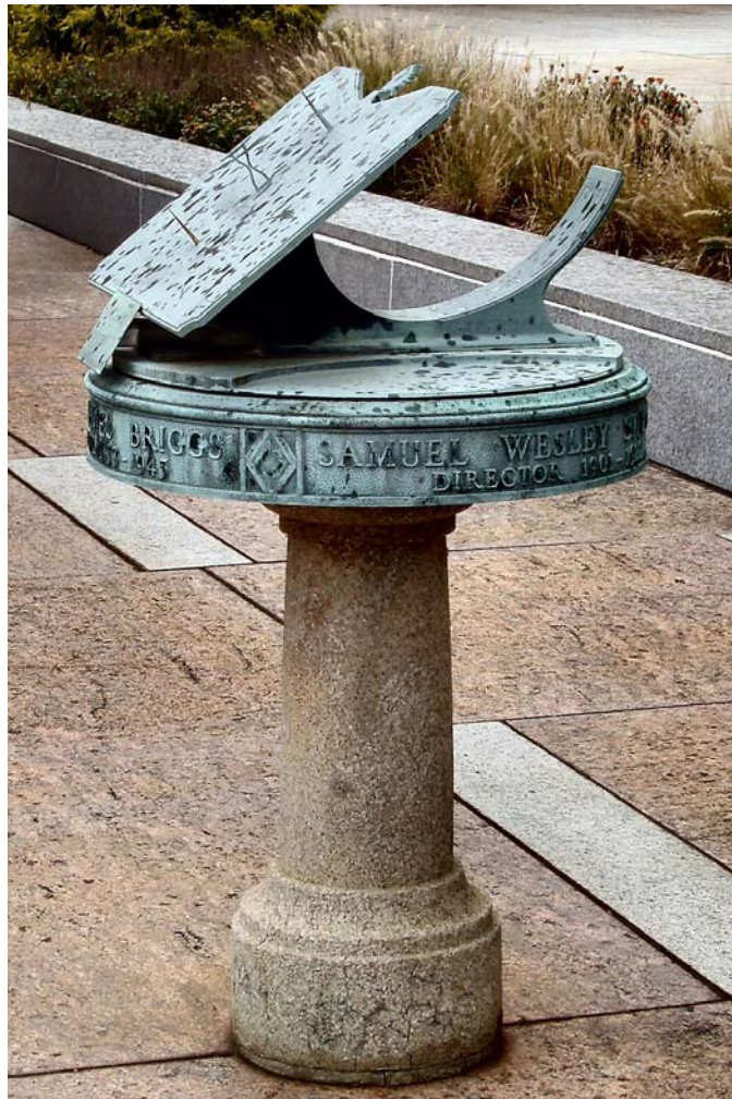
The Briggs sundial at NIST, splattered with rain drops. The lower gnomon was a temporary replacement in anticipation of our visit. The curved back portion of this polar dial carries an analemma for noon.
