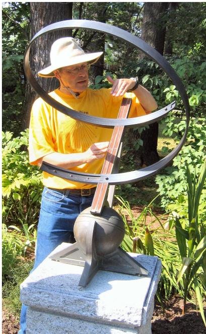
*Renaissance Sundial:* The first sundial on display was Bill’s Renaissance design, a spiral sundial that used curved mirrors to show two bright bands on the inside of the spiral. The center dark line can show the solar time to within seconds. The Renaissance dial is one of Bill’s custom Precision Sundial designs.
